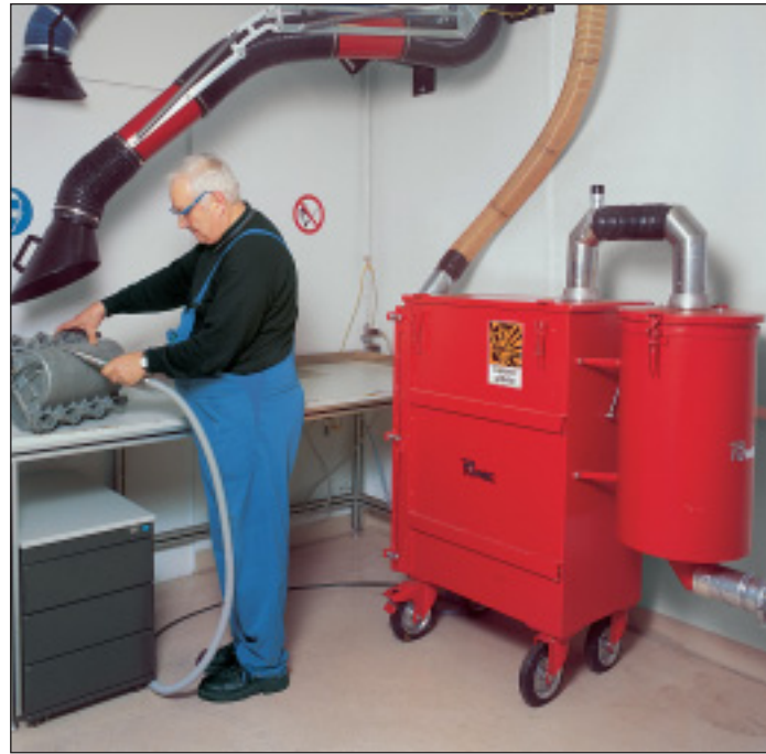
NA 250 type III with residual dust filter in normal steel
